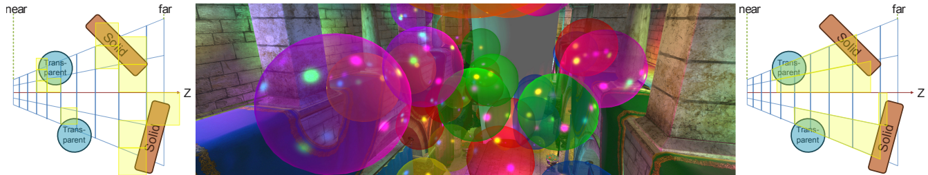
Figure 1: Shot from the Crytek Sponza scene with semi-transparent bubbles added, lit by 1024 random lights. With 8x MSAA at 720p resolution, Tiled Deferred runs at 53 FPS (without bubbles), Tiled Forward at 52 FPS and Clustered Forward at 161 FPS on a GTX 680. The diagrams illustrate how transparent geometry affects clustered and tiled forward shading.
